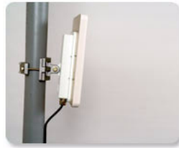
Figure 1-8: ODU with integrated Flat Panel antenna
