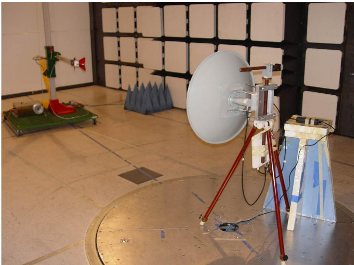
Transmitter Radiated Spurious Emissions above 1 GHz – Antenna NA
