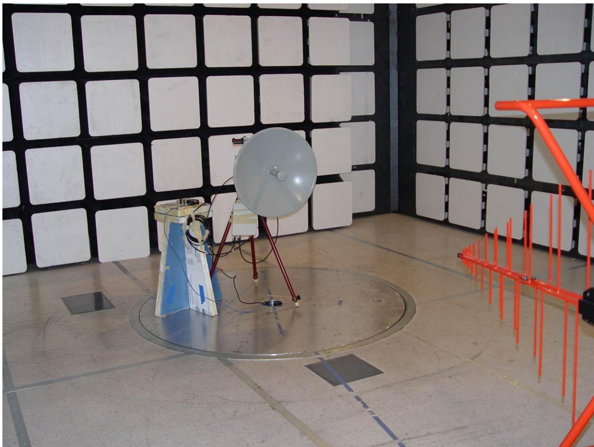
Transmitter Radiated Spurious Emissions above 1 GHz – Antenna
