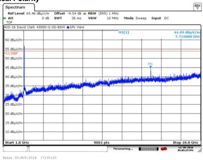
**Note:** Notch Filter used at the fundamental frequency.
