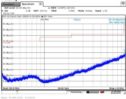
Note: Prescan from Compact 3 Meter Chamber, no Measurable signals on 3 Meter OATS.
