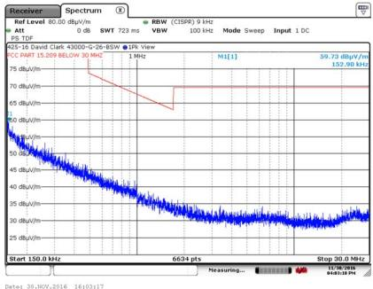
6.9.6. Antenna Perpendicular to the Device Under Test
