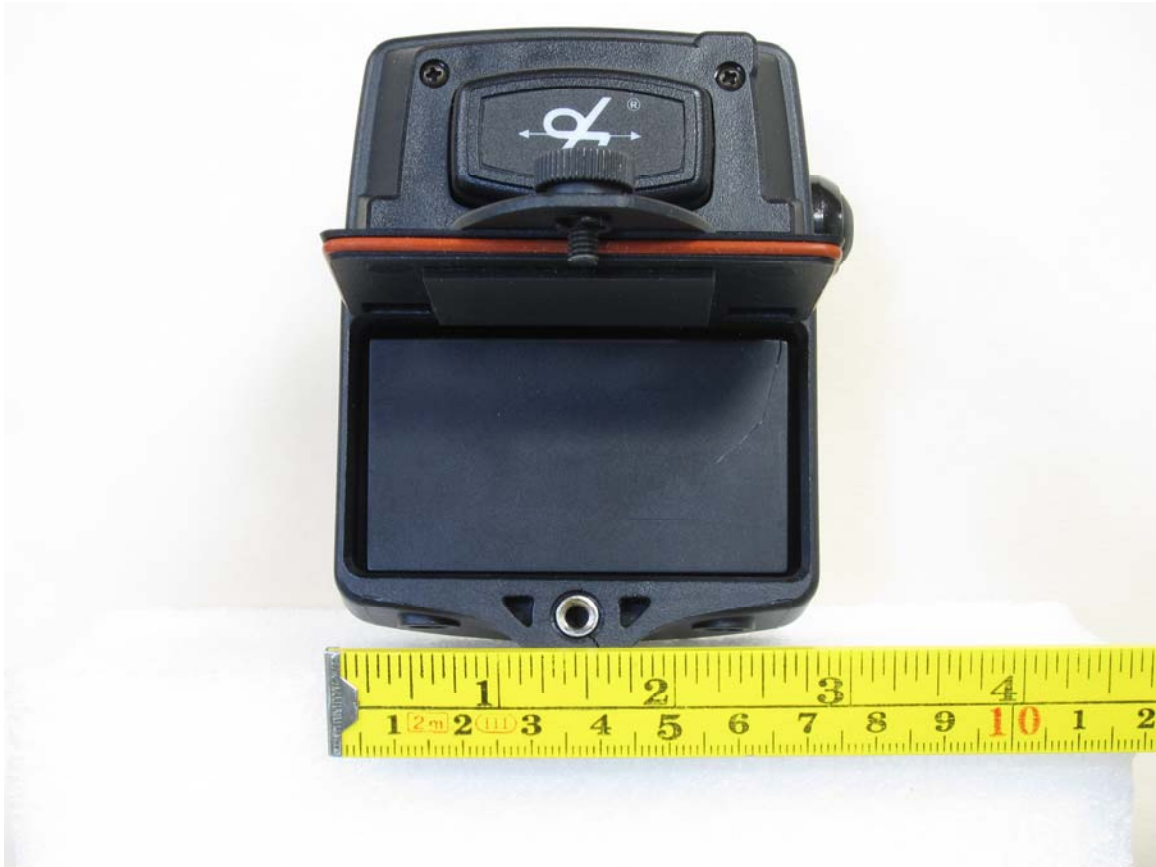
Battery Access Door Open (Battery in)
