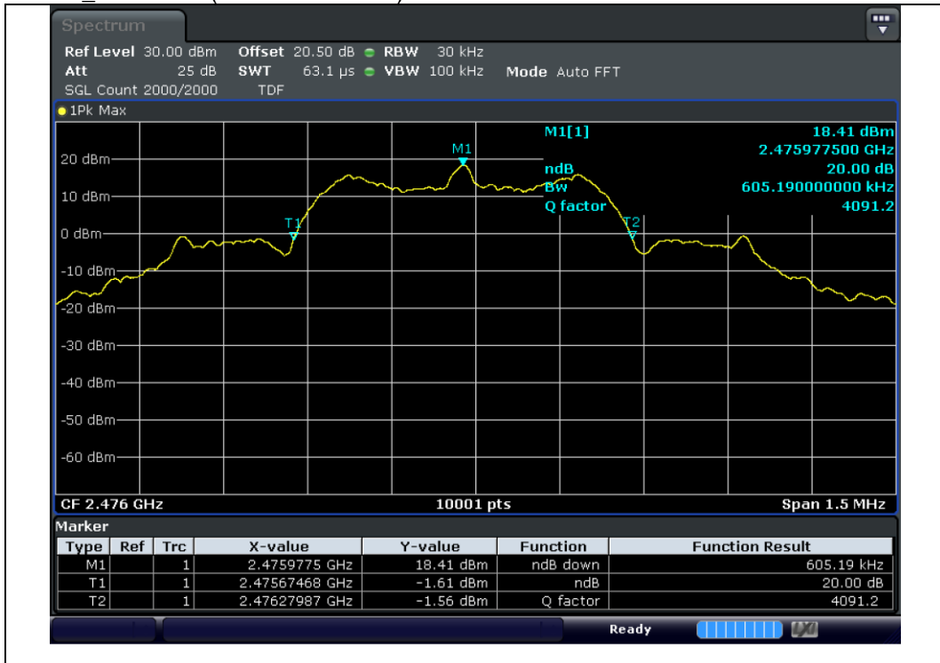
GFSK_2 476 MHz(20 dB Bandwidth)
