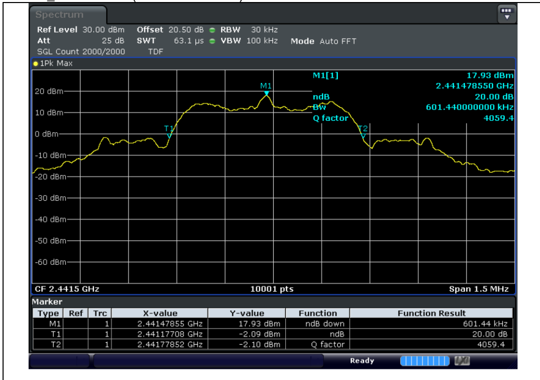
GFSK_2 441.5 MHz(20 dB Bandwidth)
