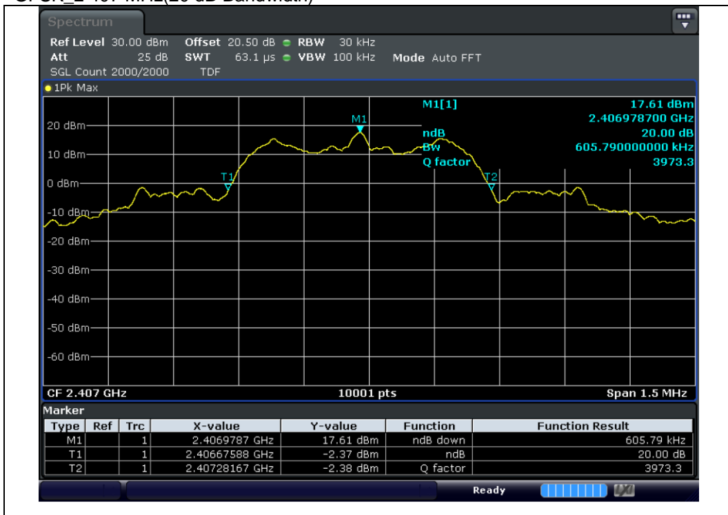
GFSK_2 407 MHz(20 dB Bandwidth)
