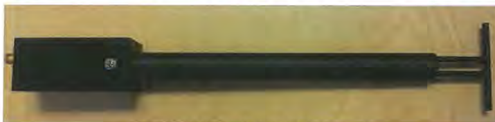
Figure 1 – MVG COMOSAR Validation Dipole
