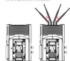
2. Please place the receiver at a height of around 1.5 to 2 meters above floor. Receiver can be placed in vertical or horizontal positions, and can be fixed via the screw at the bottom or V-mount at the back. Please install the affiliated metal stand before placing the receiver in vertical position.
