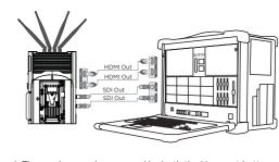
4. The receiver can be powered by both the V-mount battery and DC-IN port via the affiliated power adapter. If the mentioned two types of powersupply are connected at the same time, the lithium battery should be prioritized in power supplying, and the battery will switch to the power adapter for power supplying automatically after the battery power is exhausted.
