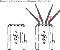
2. Please fix the transmitter via the screw at the bottom or the V-mount at the back, and place it at a height of around 1.5 to 2 meters above floor. Please make sure that the distance between each transmitter is more than 1 meter.
