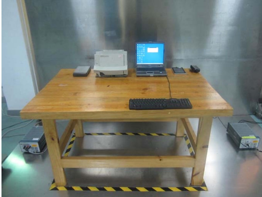
Conducted Emissions - Front View (USB Downloading)
