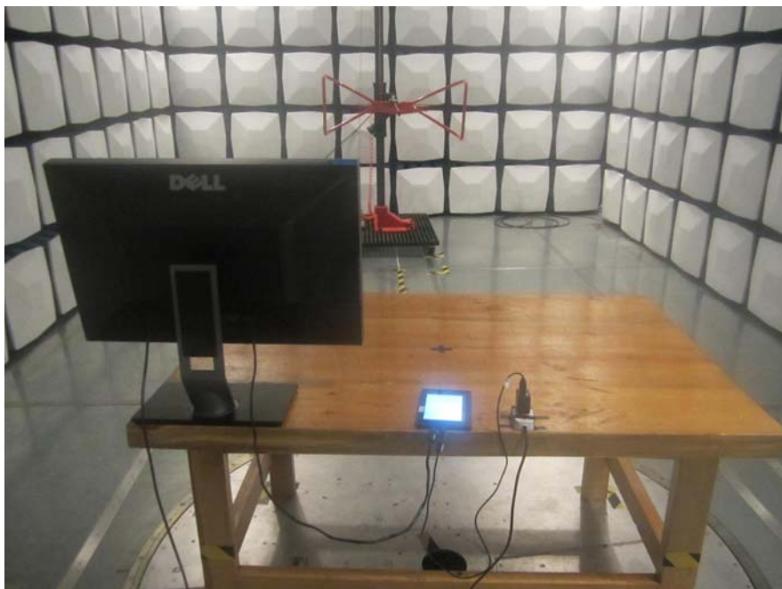
Radiated Emission - Rear View (HDMI Playing) (Below 1GHz)
