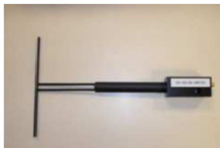
Figure 1 – Satimo COMOSAR Validation Dipole
