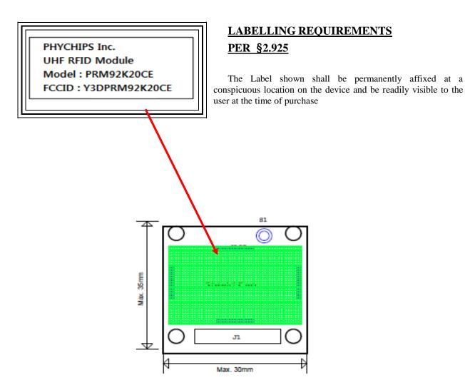
The label is attached to this device by an adhesive. The adhesive is permanent type with strong strength.
