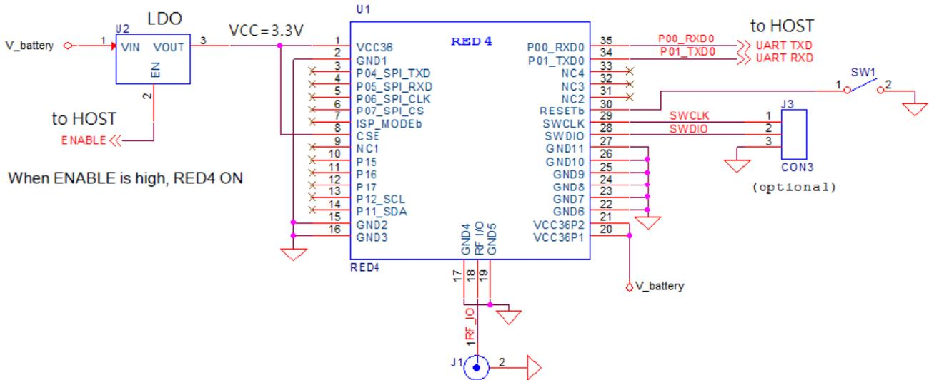
**Figure 2 Application Circuit**
