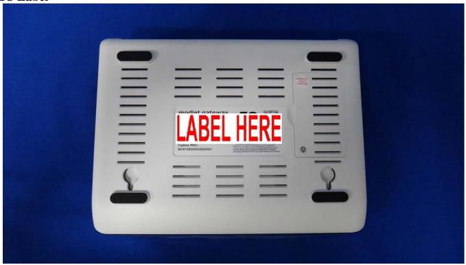
The IC Label will be placed on the equipment as shown in the photograph below.
