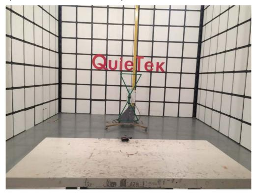
Description: Radiated Emission Test Setup for 1~18GHz
