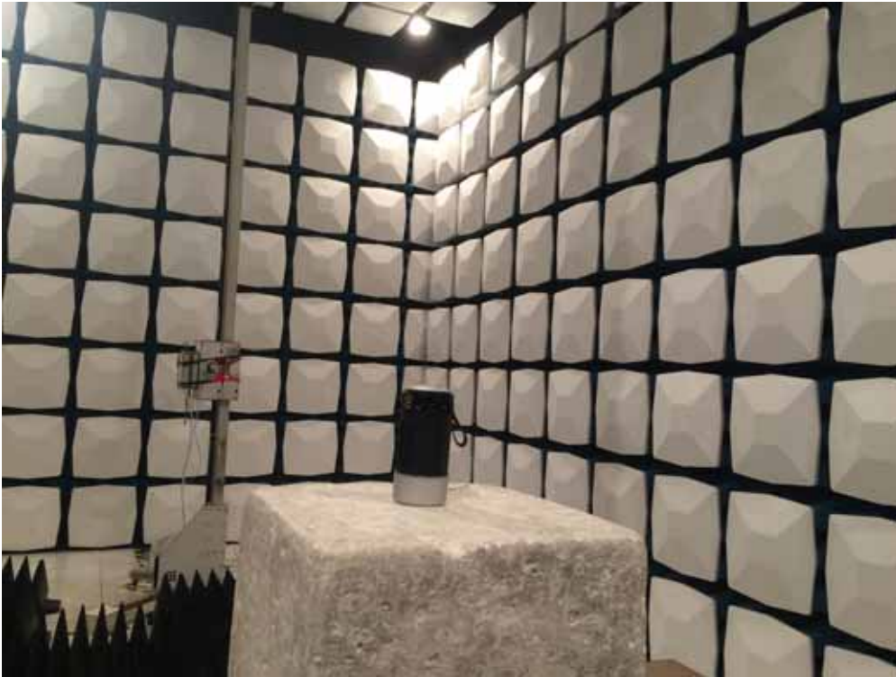
Description: Radiated Emission Test Setup for 1~18GHz
