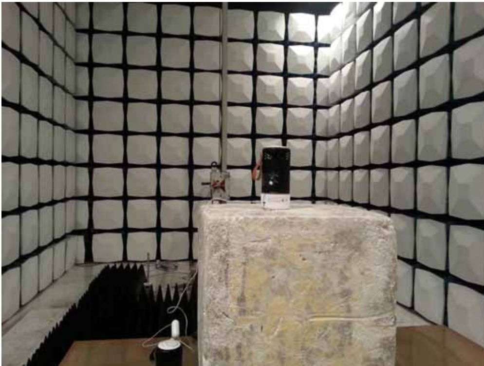
Description: Radiated Emission Test Setup for 1~18GHz
