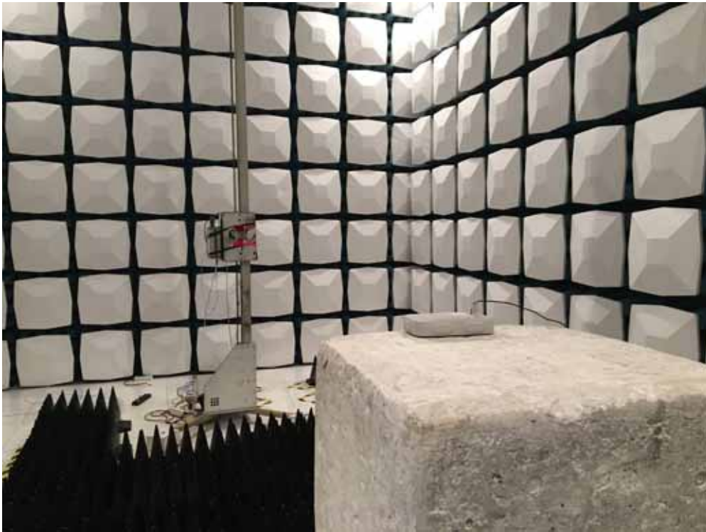
Description: Radiated Emission Test Setup for 1~18GHz
