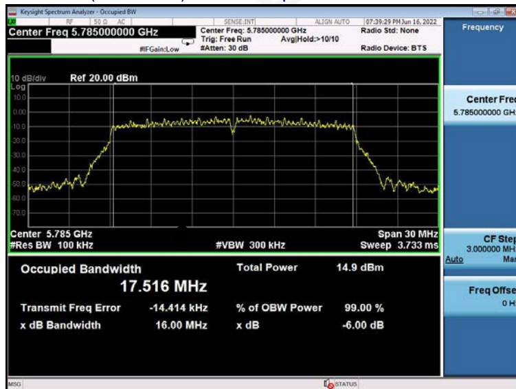
(802.11n20) Bandwidth plot on channel 165
