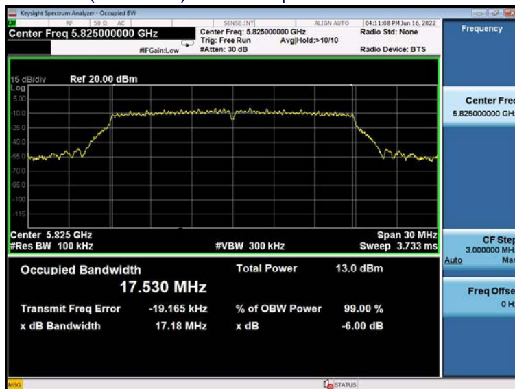
(802.11n20) Bandwidth plot on channel 165
