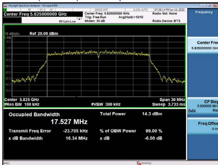
(802.11n20) Bandwidth plot on channel 165
