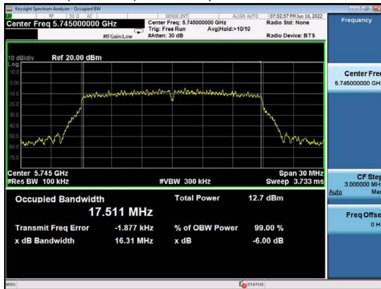
(802.11n20) Bandwidth plot on channel 157
