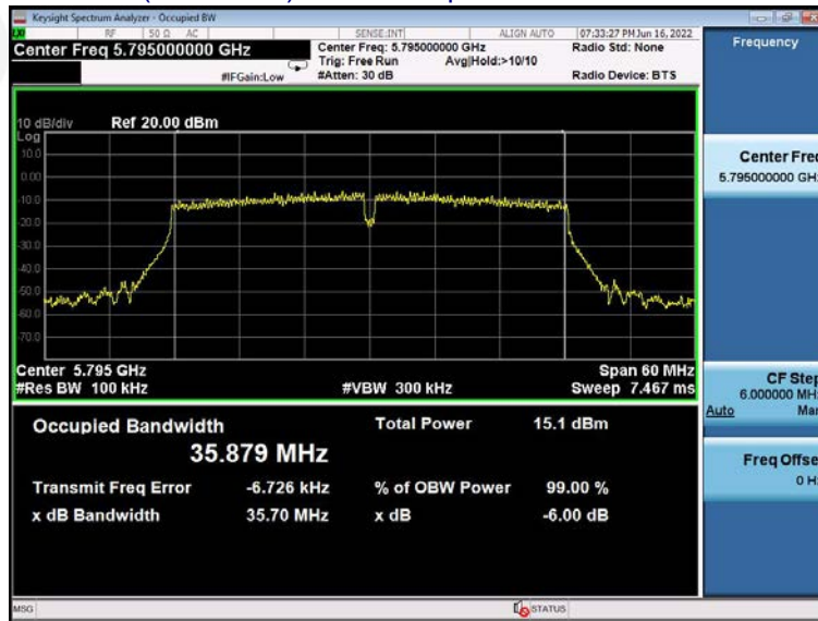
(802.11ac80) Bandwidth plot on channel 155
