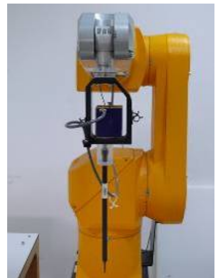
Figure 3. EX3DV4 E-field probe
