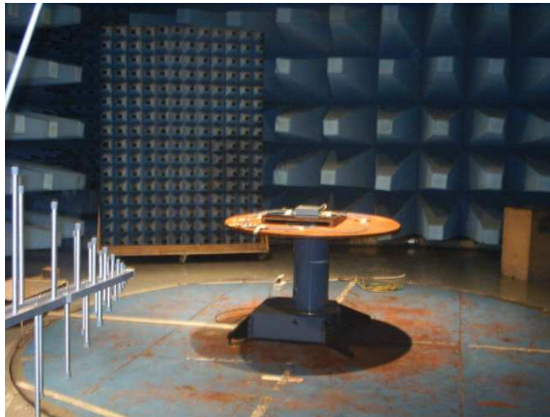
Log periodic antenna (30MHz ÷ 1000 MHz) measurement distance: 3 m
