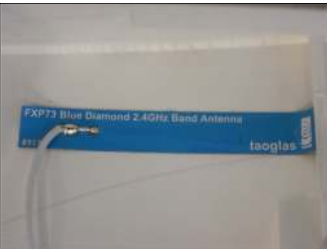
External antenna replacing the antenna integrated on the module
