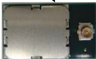
RF Module (and relevant labelling) Already FCC certified FCC ID:Y2K-PROTUBE001
