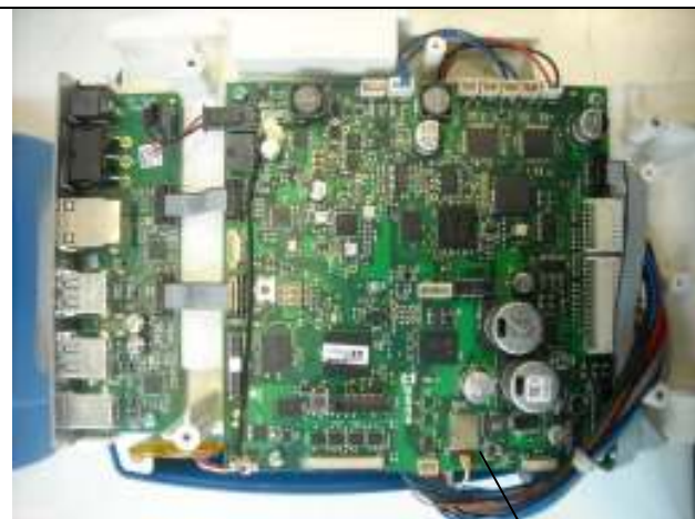
Position of RF module inside host
