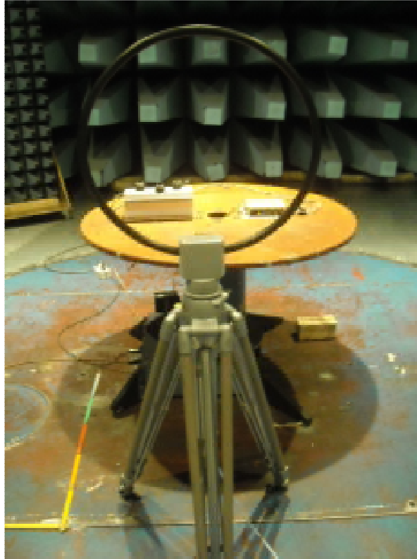
Loop antenna Rohde & Schwarz HM 020 1 meter distance
