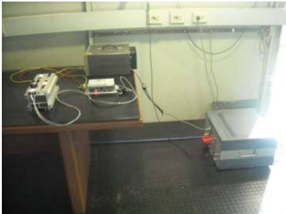
OPB by FSEK R&S + 5-1/4" loop antenna EATON model 94605-1
