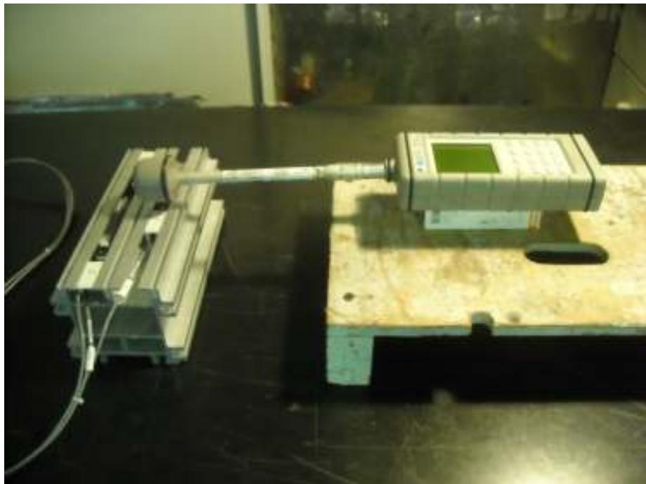
Measurement of the Magnetic Field by Loop antenna R&S model HM 020 +
