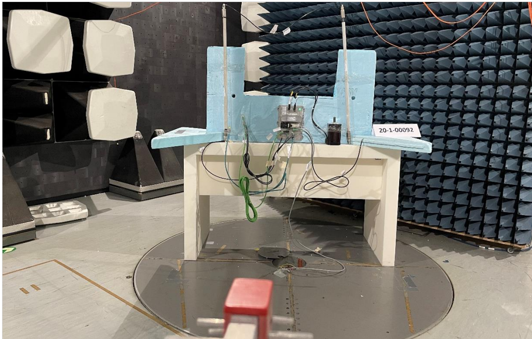
Photograph 1: EUT Test Setup in the semi anechoic chamber, Radiated interference field strength
