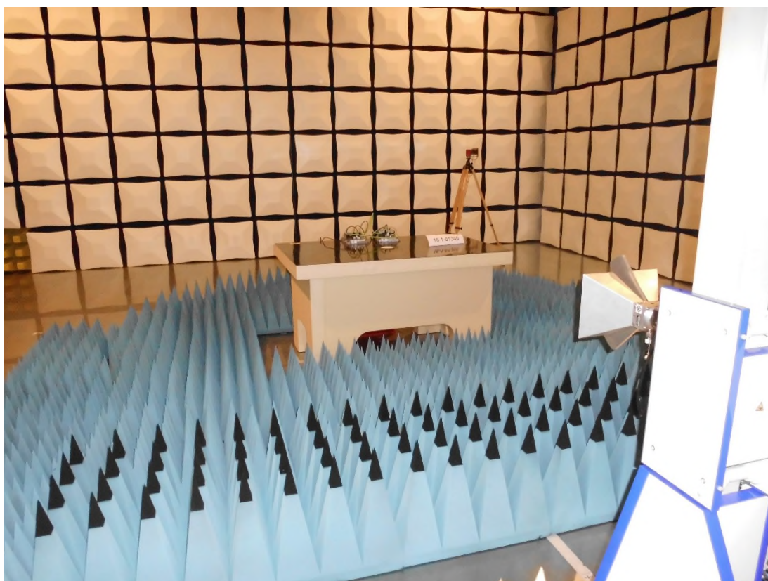
Photograph 6: Radiated emission measurements test set-up for measurement of frequency above 1000 MHz with SEW Eurodrive antenna Front side view
