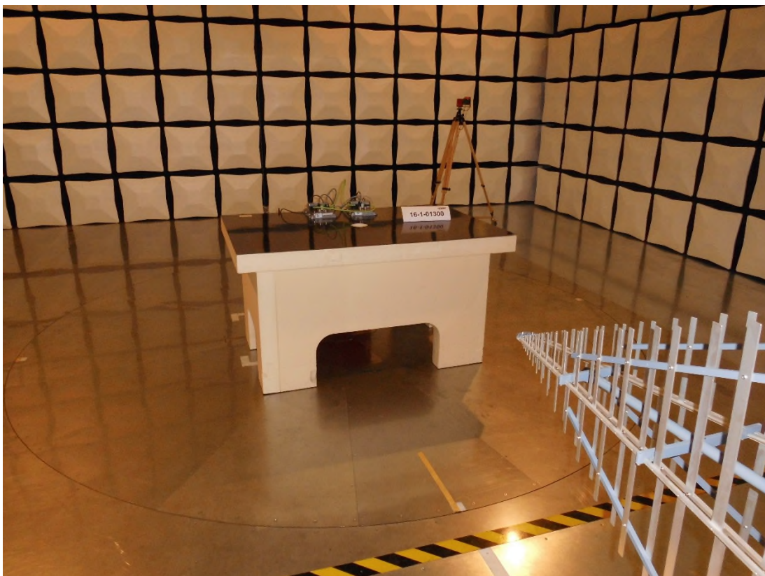
Photograph 2: Radiated emission measurements test set-up for measurement of frequency up to 1000 MHz with SEW Eurodrive antenna Front side view
