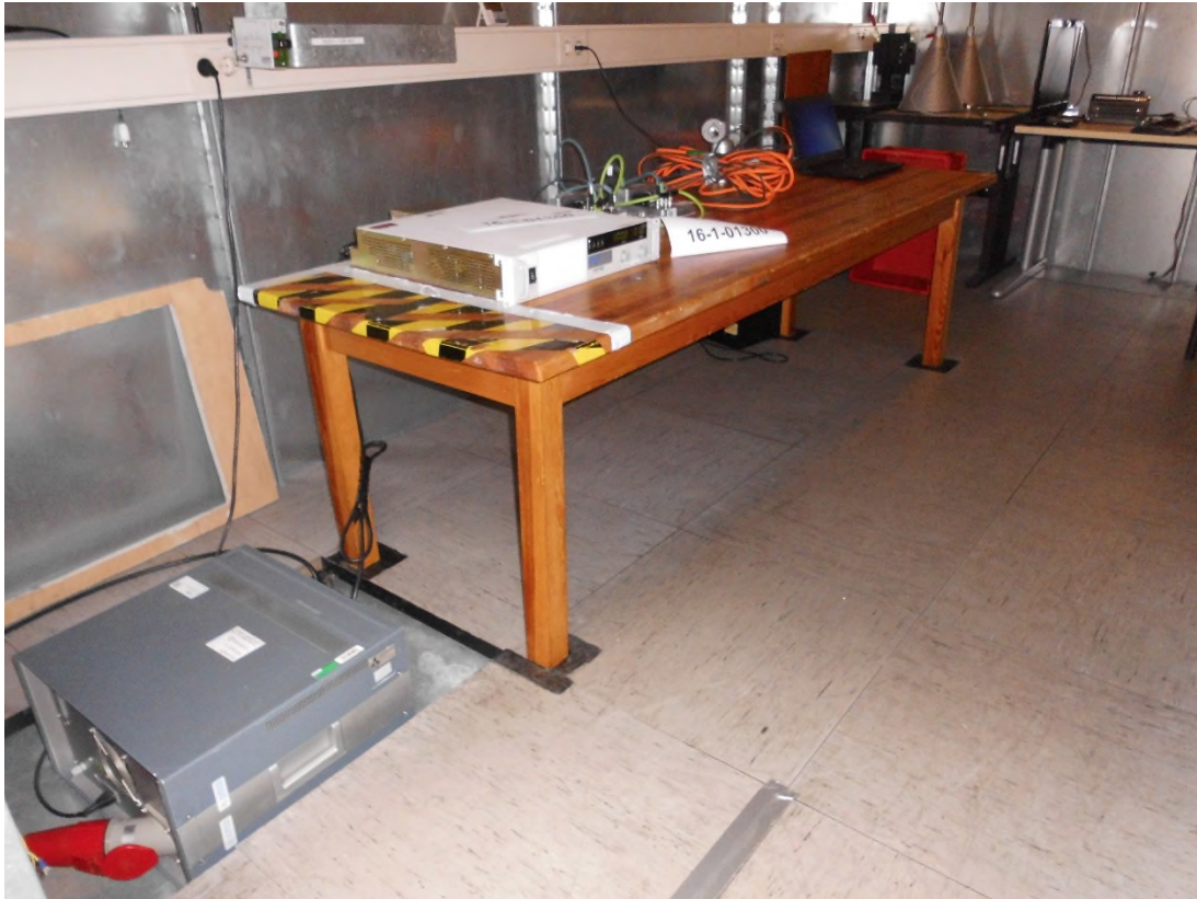
Photograph 1: Mains conducted emission measurements test set-up for measurement of frequency up to 30MHz
