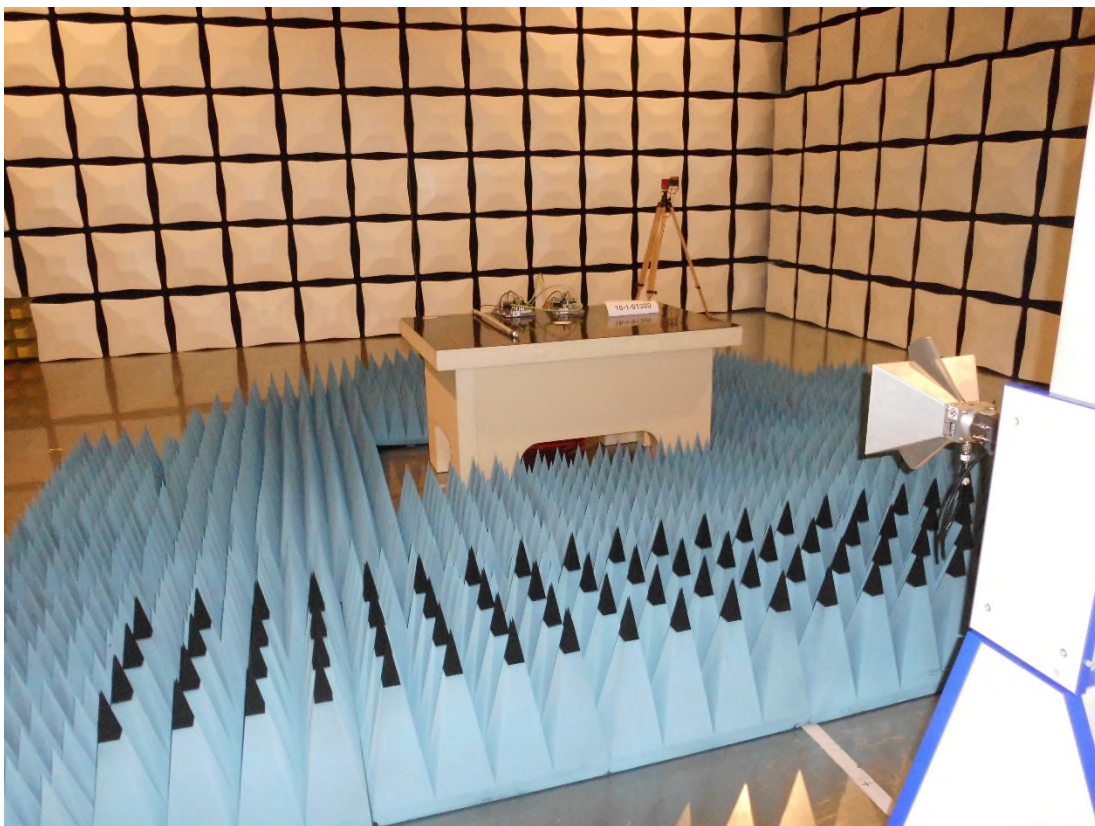
Photograph 8: Radiated emission measurements test set-up for measurement of frequency above 1000 MHz with rod antenna Front side view
