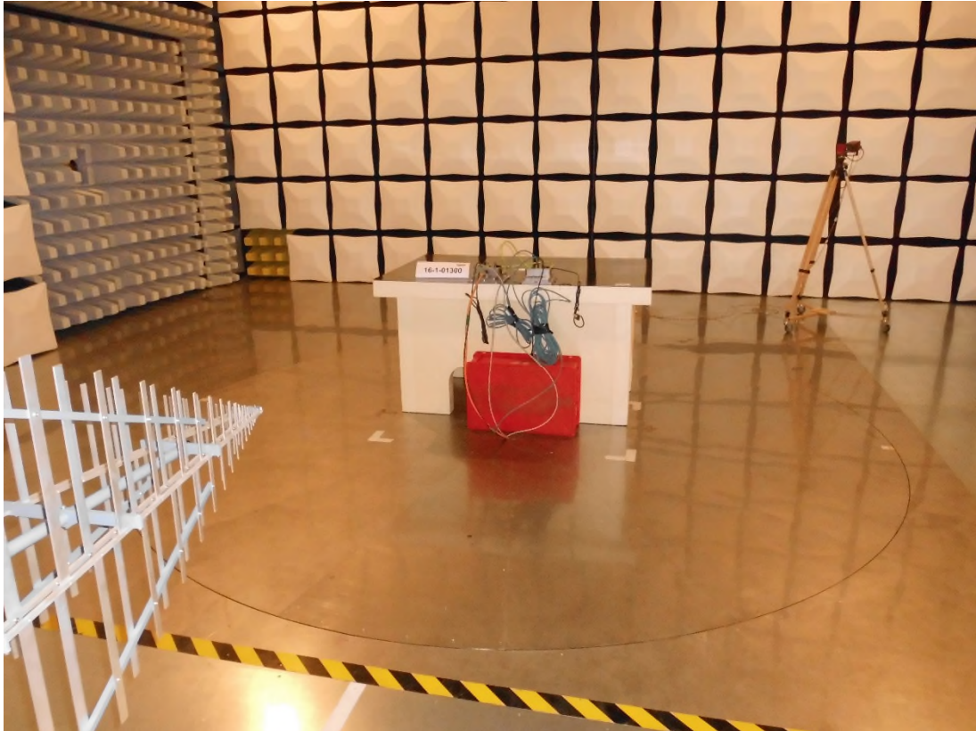
Photograph 3: Radiated emission measurements test set-up for measurement of frequency up to 1000 MHz with SEW Eurodrive antenna Rear side view
