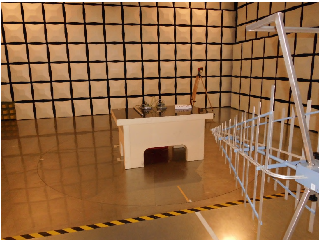
Photograph 4: Radiated emission measurements test set-up for measurement of frequency up to 1000 MHz with rod antenna Front side view
