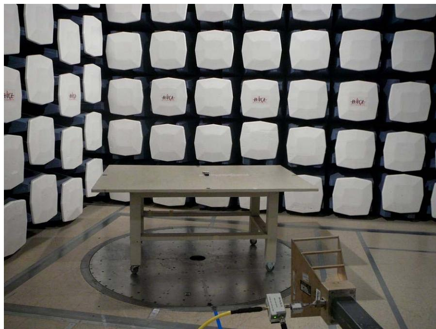
**14.4 Radiated Emission above 1 GHz Front View @ 3 Meters**
