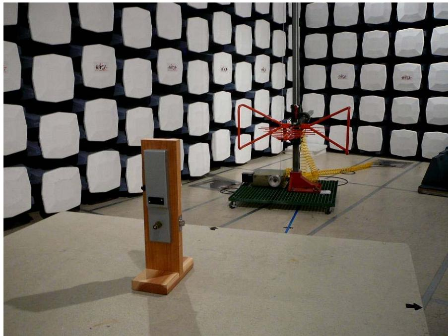
**17.3 Radiated Emission above 1 GHz Front View @ 3 Meters**
