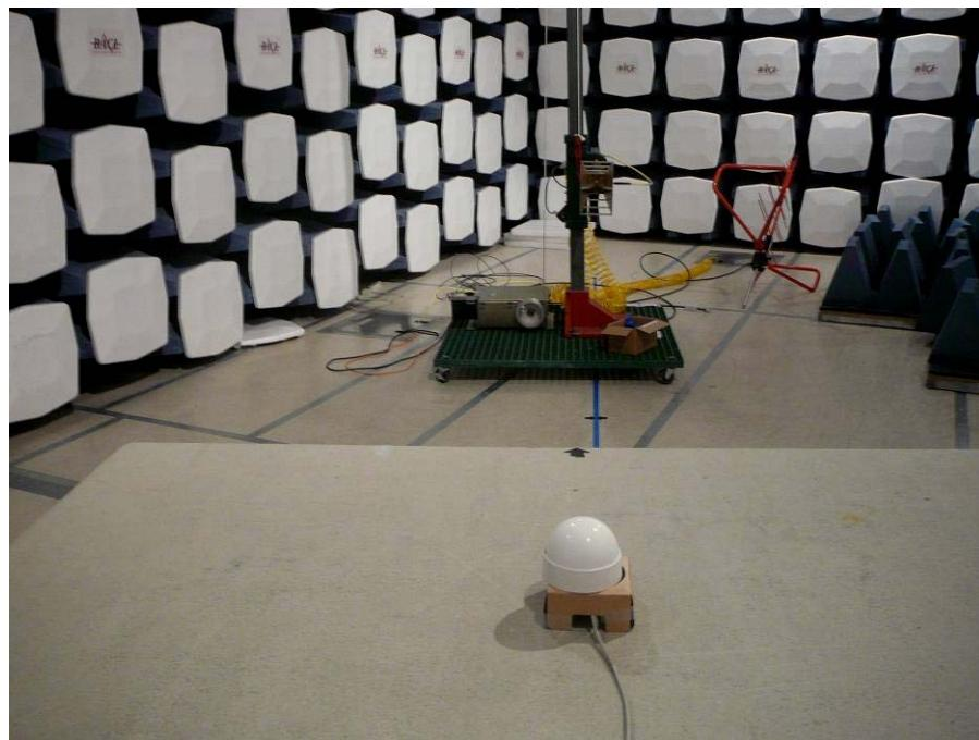
**14.5 AC Line Conducted Emission Front View - PoE**
