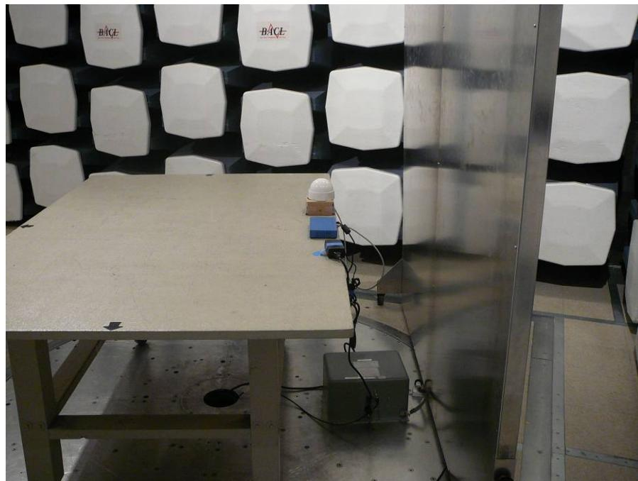
**14.7 AC Line Conducted Emission Front View – Power AC/DC Adaptor**
