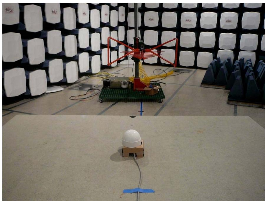
**14.3 Radiated Emission above 1 GHz Front View @ 3 Meters**
