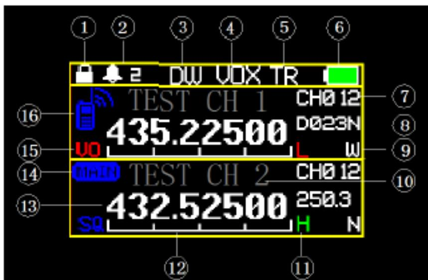
①Lock key: icon shows up, keypads are not allowed to operate; if the icon is red, which means the radio is in Remotely Stun status.
