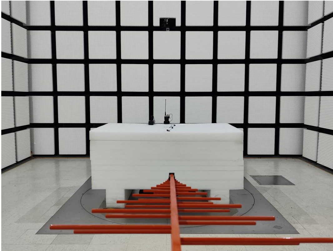
Radiated Emission Below 1GHz rear View M2
