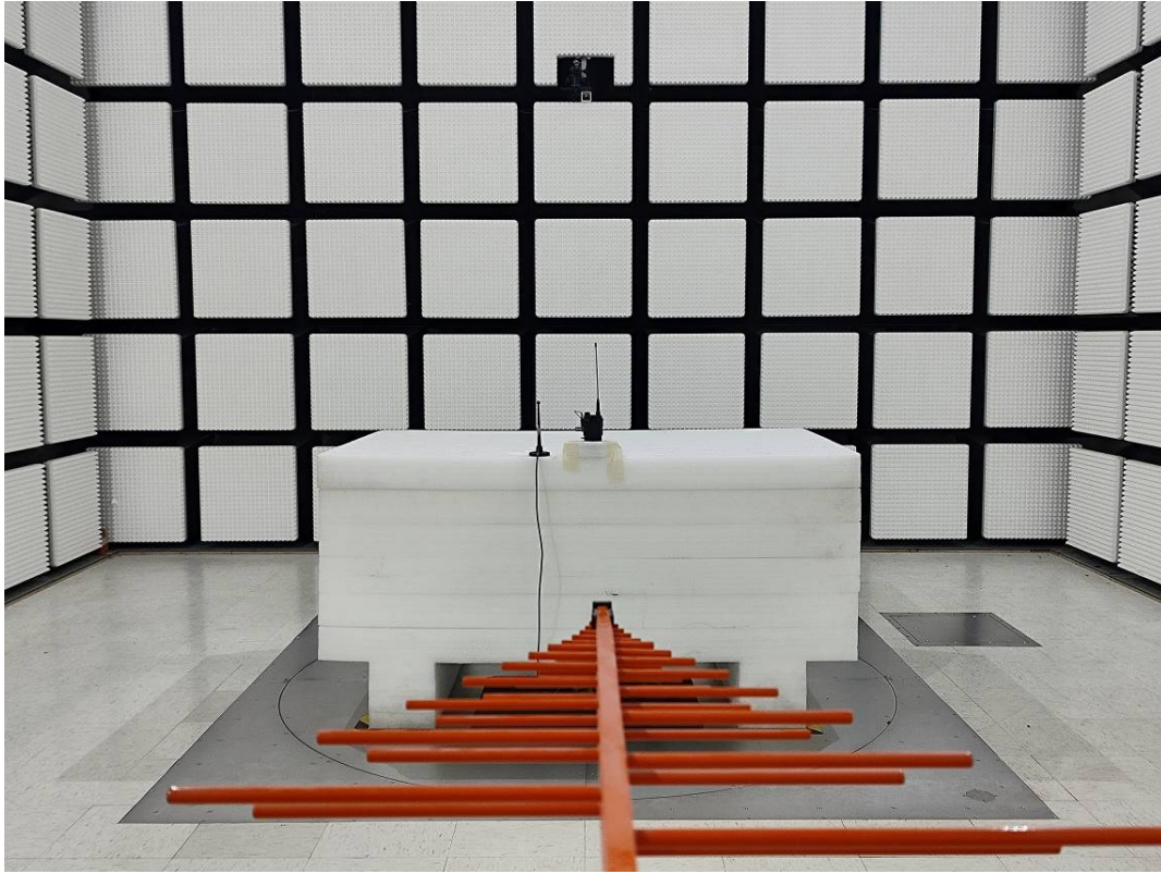
Radiated Emission Below 1GHz rear View M3-M6
