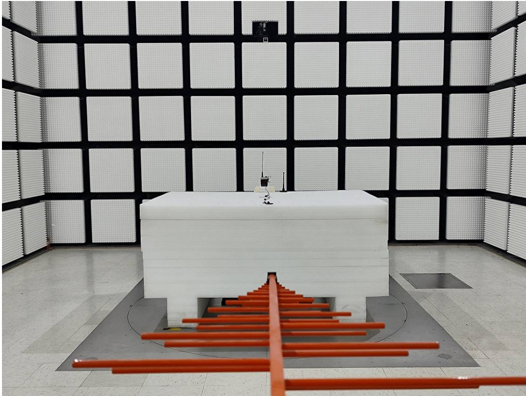
Radiated Emission Below 1GHz rear View M3-M6
