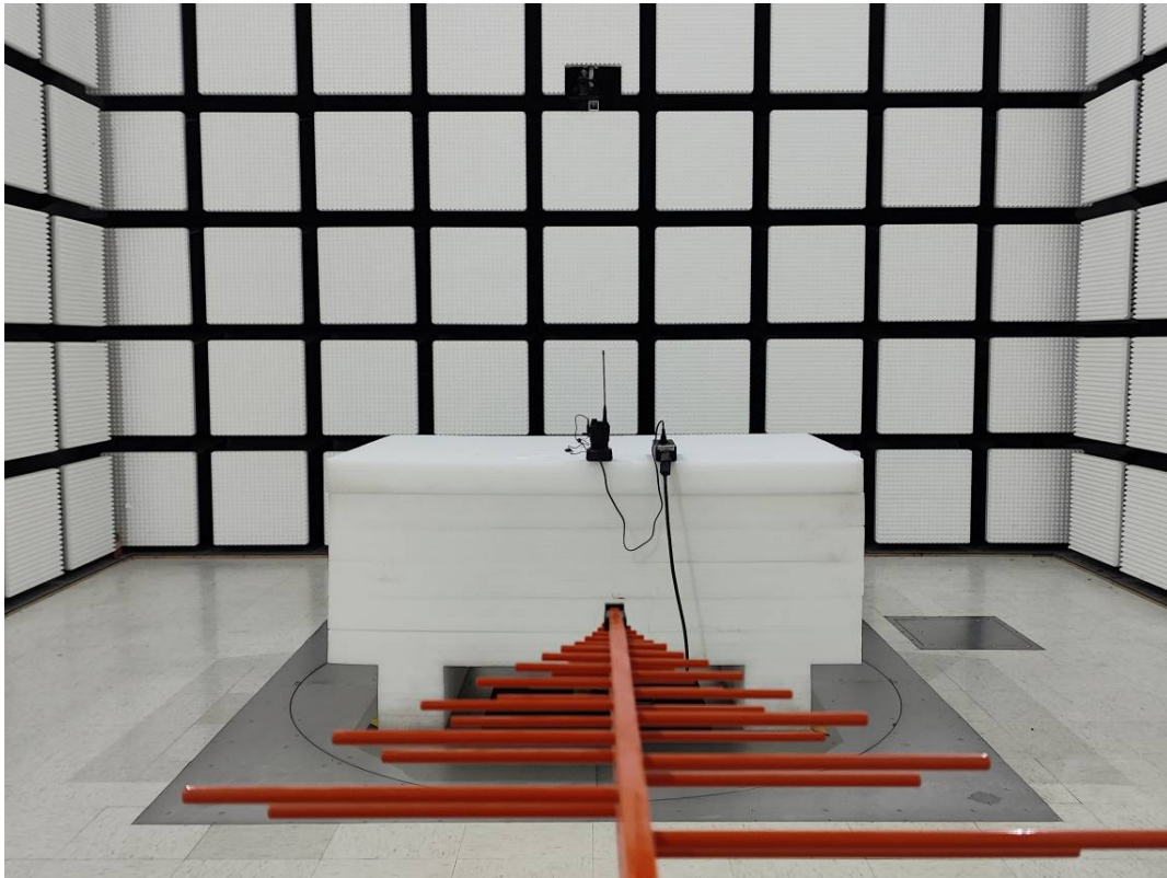
Radiated Emission Below 1GHz rear View M2
