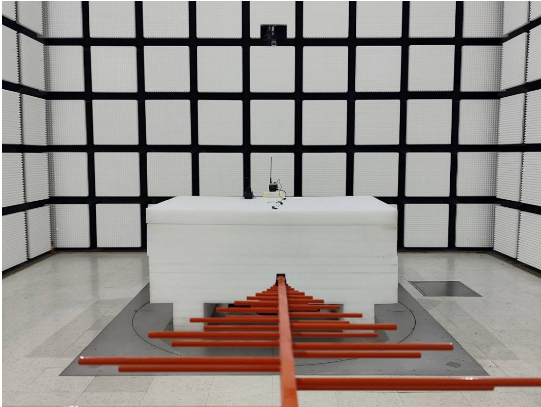
Radiated Emission Below 1GHz rear View M1
