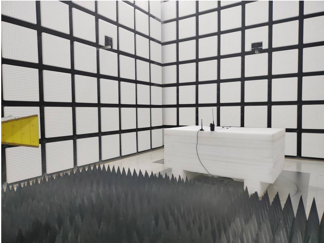
Radiated Emission Above 1GHz rear View M3-M6
