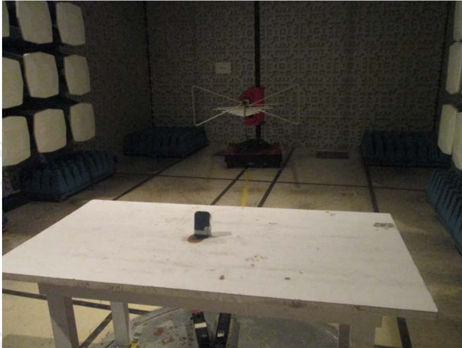
TEST SETUP OF RADIATED EMISSION (30MHz-1GHz)
