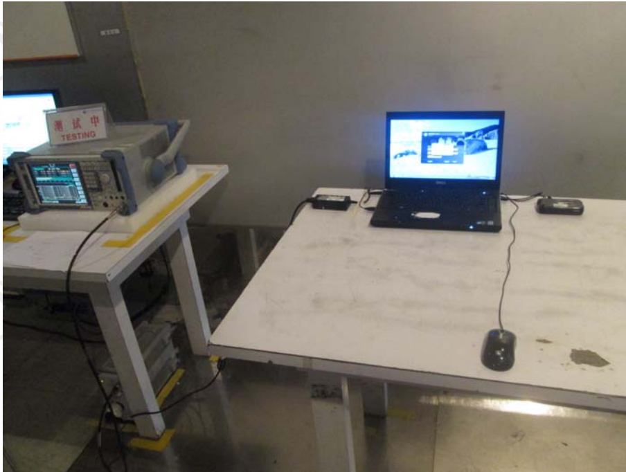
TEST SETUP OF CONDUCTED EMISSION
