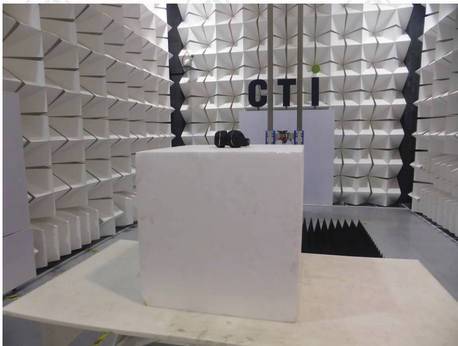
Radiated spurious emission Test Setup-2(Above 1GHz)
