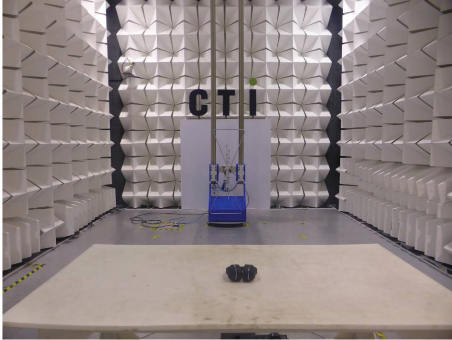
Radiated spurious emission Test Setup-1(Below 1GHz)
