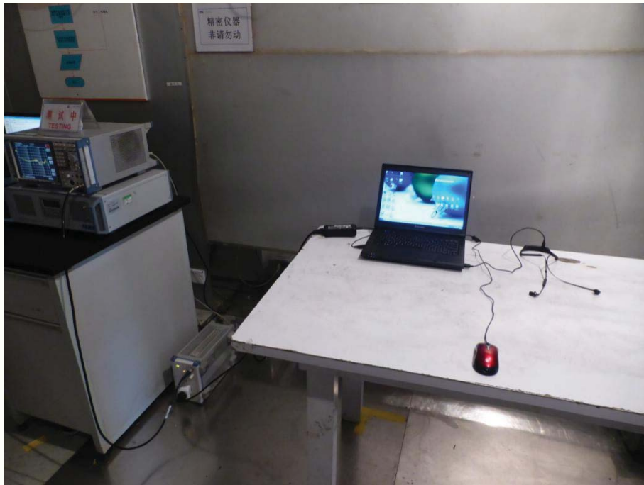
Conducted emission Test Setup
