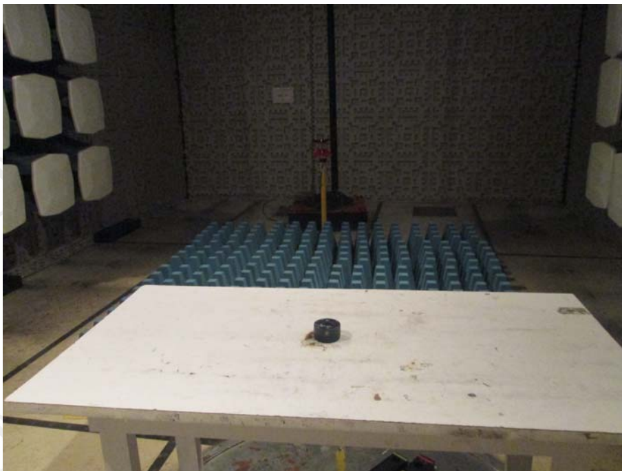
TEST SETUP OF RADIATED EMISSION (above 1GHz)
