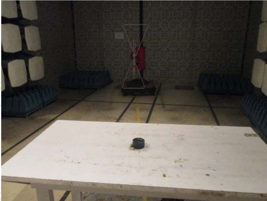
TEST SETUP OF RADIATED EMISSION (30MHz-1GHz)
