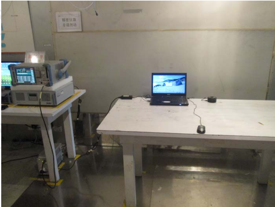
TEST SETUP OF CONDUCTED EMISSION
