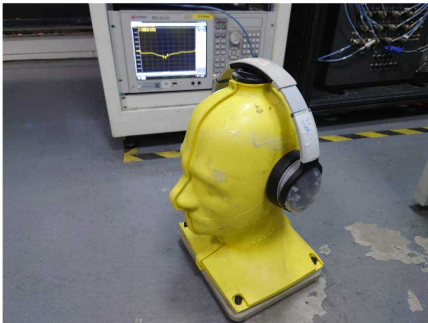
Beside Head #1 Impedance Setup
