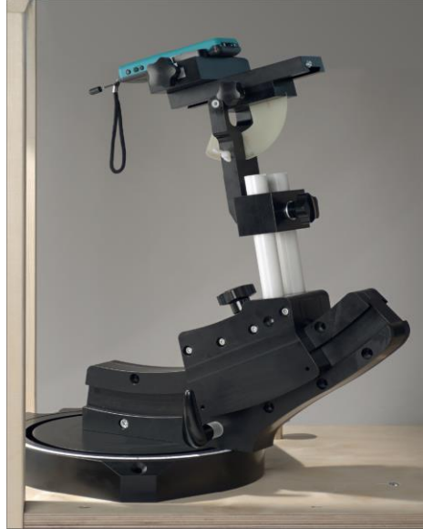
F-2. Device Holder for Transmitters
