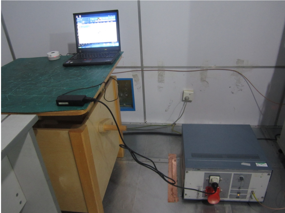
Conducted Emission Test setup photo
