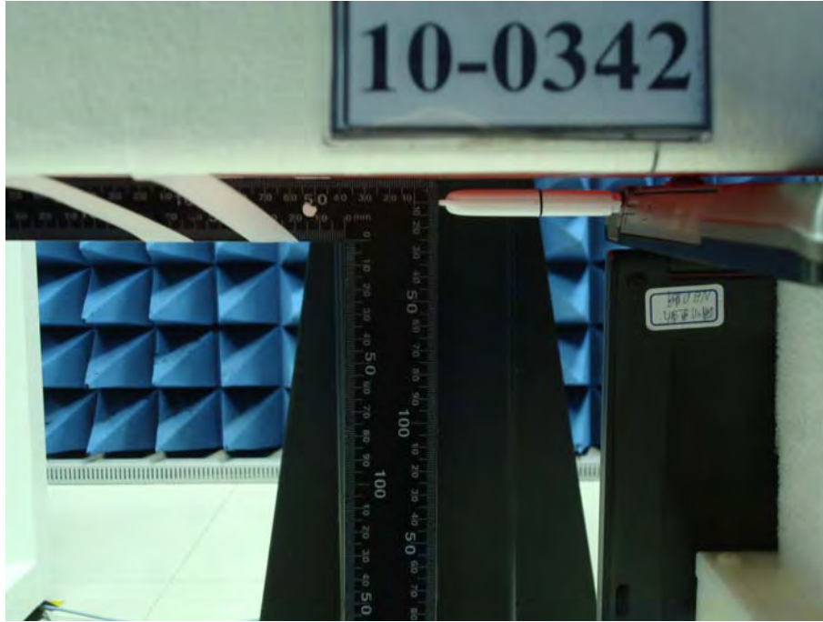
Figure 1. Horizontal Up, EUT to Phantom 5mm space _ LCD Open90 degree
