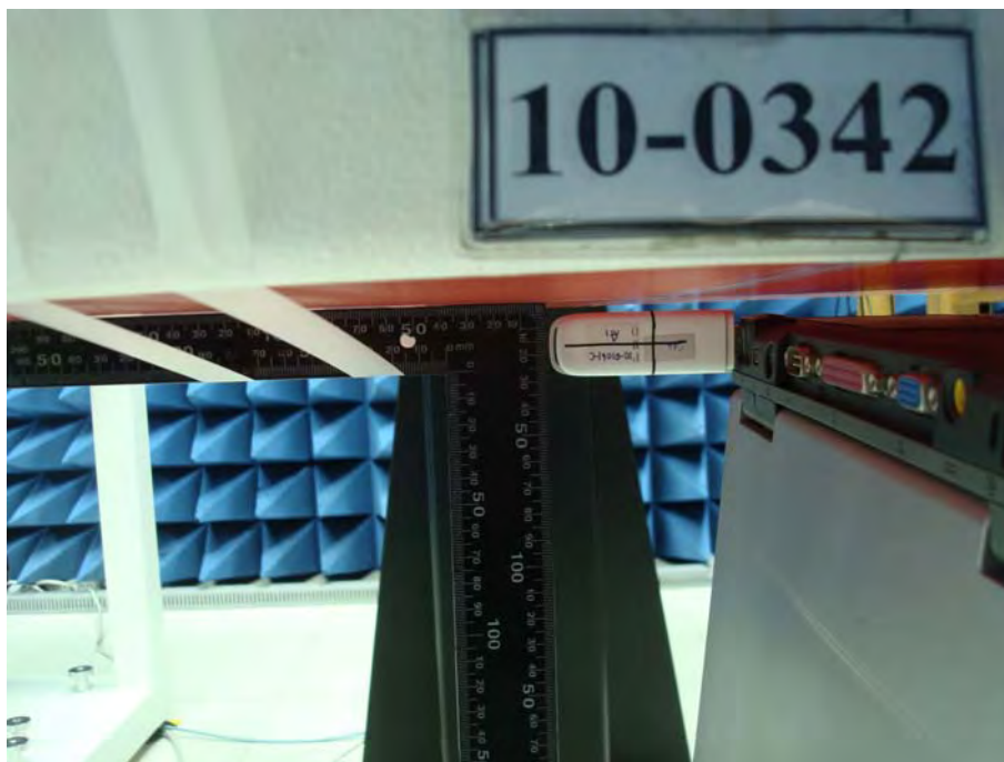
Figure 5. Vertical Front, EUT to Phantom 5mm space _ LCD Open90 degree
