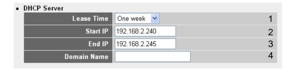
These settings are only available when 'DHCP Server' in 'LAN IP' section is 'Enabled', and here are descriptions of every setup items:
