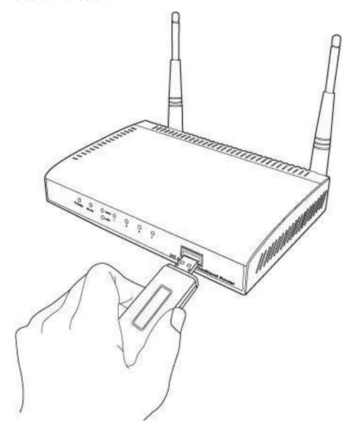
2. Connect your xDSL / cable modem to the WAN port of router by Ethernet cable.
