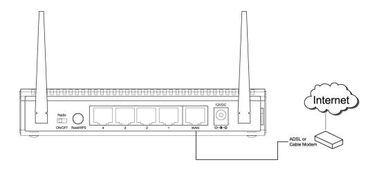
3. Connect all your computers, network devices (network-enabled consumer devices other than computers, like game console, or switch / hub) to the LAN port of the router.
