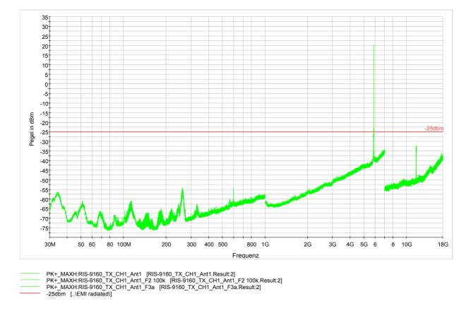
Although the measurement above ends at 18 GHz, radiated measurements were made up to 40 GHz, but no graph is available. No emissions above noise level were found above 18 GHz.
