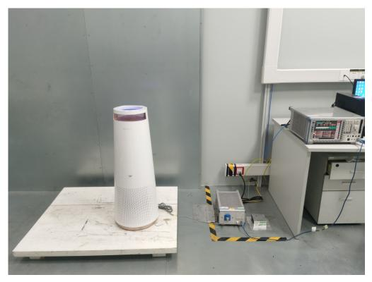
Radiated emission test 30MHz – 1GHz
