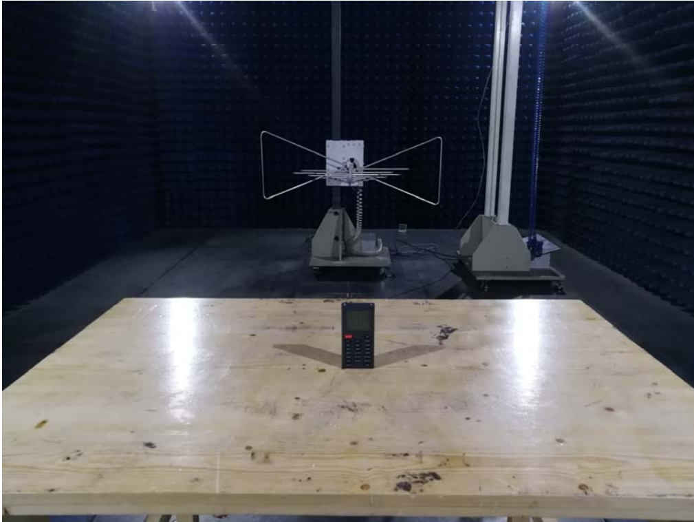
Photograph of set-up for Radiated Emission
