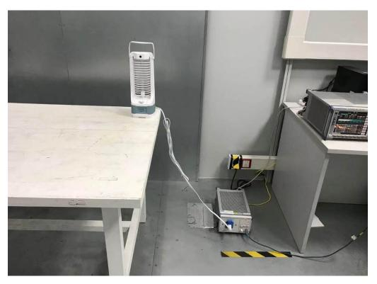
Radiated emission test 30MHz – 1GHz
