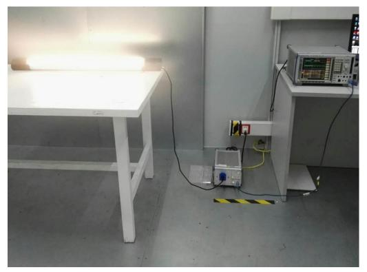
Radiated emission test 30MHz – 1GHz
