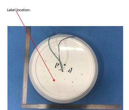
75mm Led Ceiling Lamp 54075541 AC 120V 60Hz 230mA 22W 4000K 2400Im CRI80 Made in China CAUTION-SUITABLE FOR DAMP LOCATIONS. 60mm SUITABLE FOR OPERATION IN AMBIENT NOT This device complies with part 15 of the FCC Rules. Operation is subject to the following two conditions:
