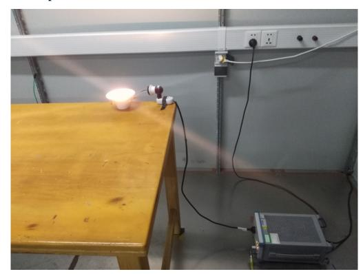
1.1. Photos of power line conducted emission test
