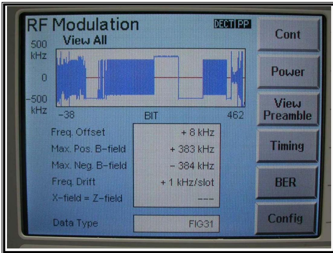
**b) Carrier Frequency Stability over temperature**
