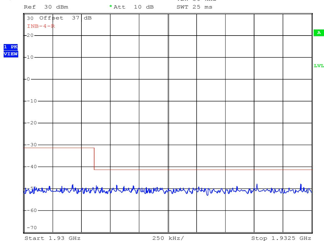
b) CH F<sub>H</sub>Out-of -band Unwanted Emission (above 1GHz): CH F<sub>H</sub>Operation Mode : TransmittingFundamental Frequency : 1928.448MHzTest Date : Jun. 19, 2011 Temperature : 25 °C Humidity : 51 %
