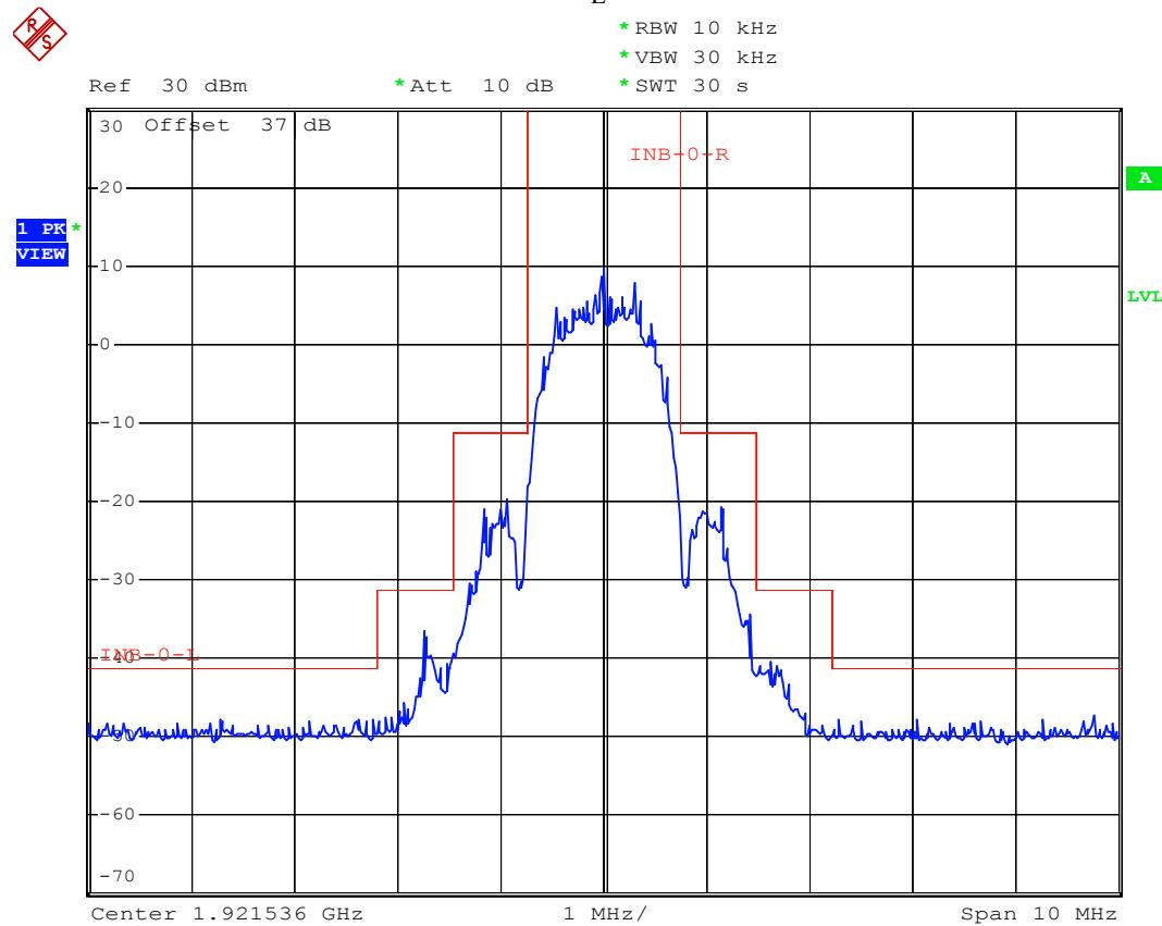
In-band Unwanted Emission: CH F<sub>H</sub>
