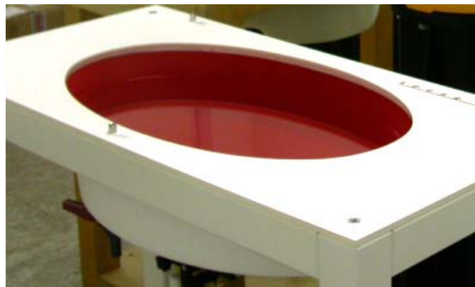
Fig. 8 SAM Twin Phantom and ELI4 Phantom
