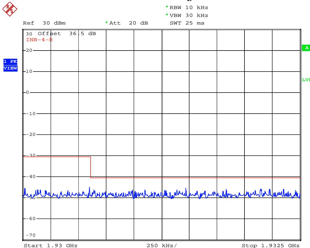
b) CH F<sub>H</sub>Out-of -band Unwanted Emission (above 1GHz): CH F<sub>H</sub>Operation Mode : TransmittingFundamental Frequency : 1928.448MHzTest Date : Jul. 04, 2010 Temperature : 23 °C Humidity : 56 %
